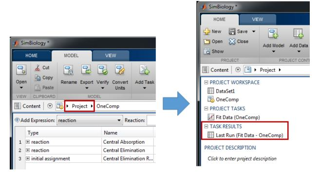
Each time you run the same fit task, this **Last Run** entry is overwritten. If you plan to run the task again and want to keep the results of the last run, save the data. Right-click on the **Last Run** entry and select **Save Data** and specify a name for the data. When you rerun the task, the results are stored in the **Last Run** entry, and your previously saved data is unchanged. Note that each task has its own **Last Run** entry.
