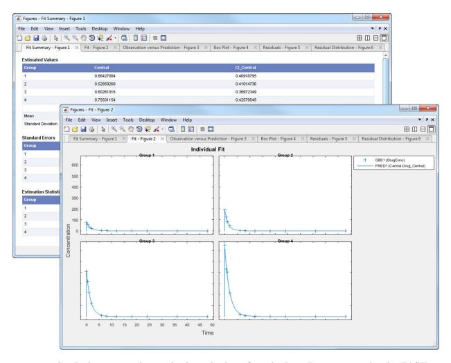
SimBiology stores the results from the fit task in the **Last Run** entry under the **TASK RESULTS** section of the Project. You can navigate to the project area by clicking the **Project** on the navigation bar of the main desktop window.
